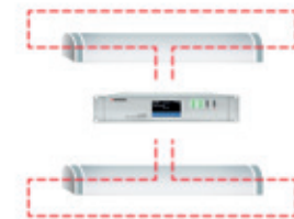
Loop, cable redundancy only
