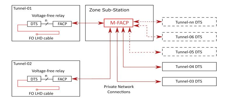
Each LHD unit has a wall mounted enclosure for easy installation on a vertical wall. In the event of a power supply interruption, each LHD unit also has a battery backup unit that ensures uninterrupted fire detection and monitoring.
