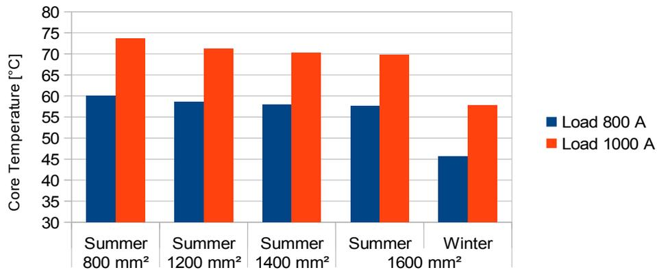
Figure 4 Simulated core temperature of the cable considered for installation according to IEC 60287
