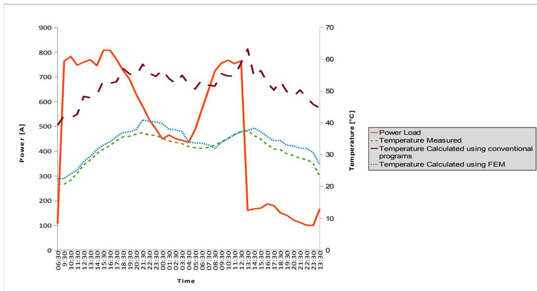
Figure 9 Load carrying over one day. Outside Temperature around 0 °C
