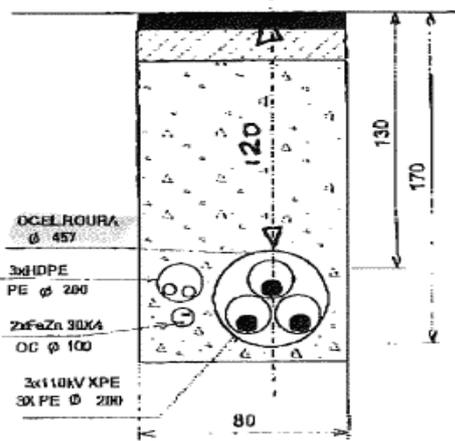
Figure 7 Laying below the rail road
