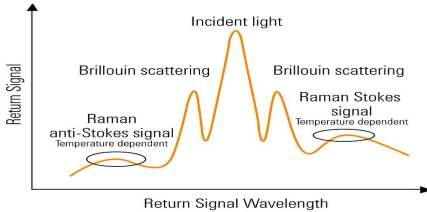
Figure 1 Incident light, Raman and Brillouin scattering over the frequency band
