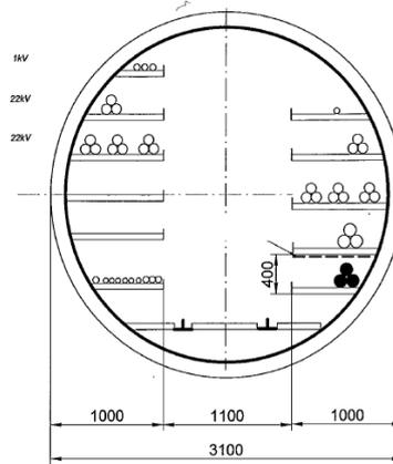
Figure 8 Tunnel Dimensions
