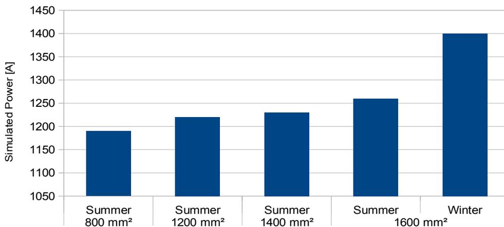
Figure 5 Simulated power transmission of cable laid in earth taking the heat pipeline influence into account
