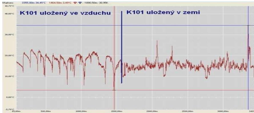
Figure 6 Diagram of temperature measured on the 17.02.2010. load about 800 A, ambient temperature around 0°C
