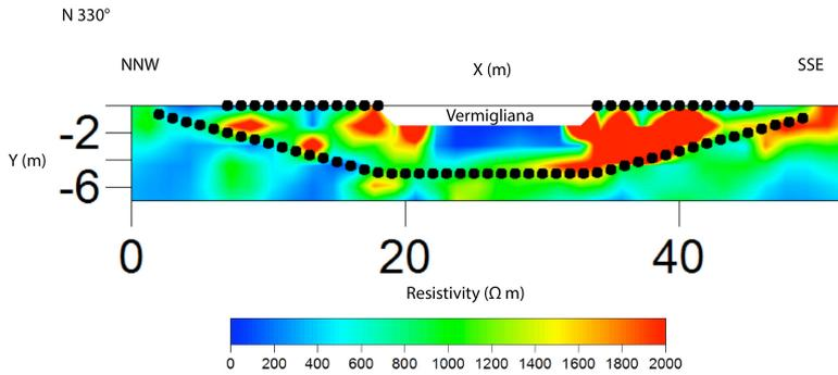
**Fig. 1.1** Example of resistivity cross-section resulting from the ERT survey conducted in Vermiglio on 20th June 2014. The cross-section is facing downstream. A low resistivity domain is located under the Vermigliana creek, while the riparian zones show, on average, higher resistivity values. The black dots represent the electrodes position both on the levee surface (24 stainless steel electrodes) and inside the perforation drilled under the Vermigliana creek (48 brass electrodes)
