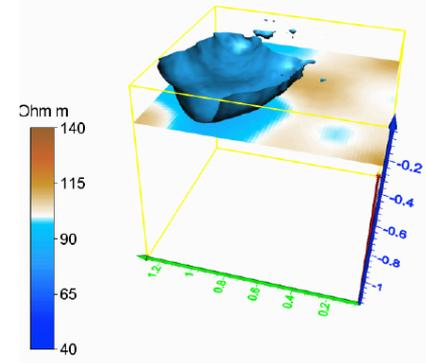
**Fig. 1.3** Isosurface representing the injection plume in the irrigation test in Bulgherano, at the first time step of the time-lapse 3D micro-ERT monitoring. The values are expressed as resistivity ratio percentages with respect to the background survey.
