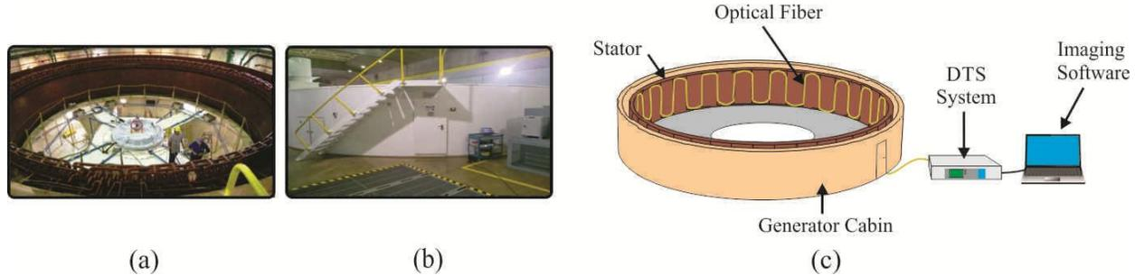
Fig. 1. Overview of the methodology used in the experimental tests with the thermal imaging system. (a) Picture of generator stator. (b) Picture of generator cabin and imaging system. (c) Schematic with components involved.
