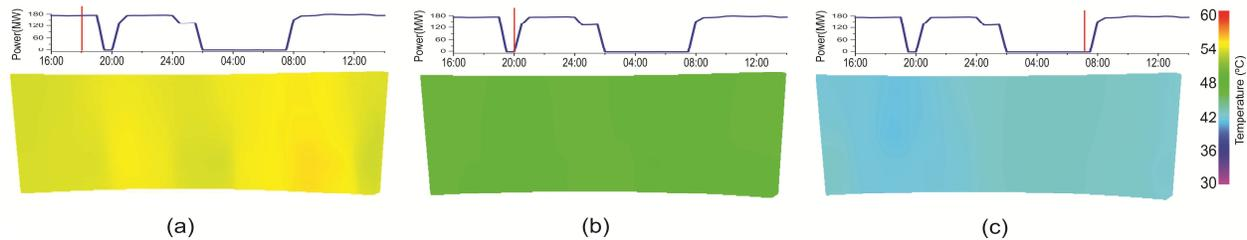
Fig. 4. (a) Thermal image during normal operation of the generator, where the average temperature is 54 °C. (b) Thermal image after 1 hour operating without load, where the average temperature is 45 °C. (c) Thermal image after 7 and a half hours operating without load, where the average temperature is 41 °C.
