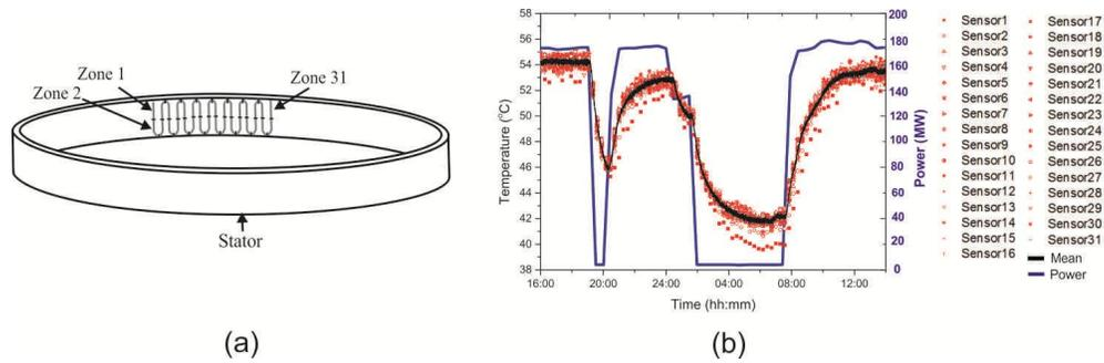
Fig. 3. (a) Scheme used for the installation of optical fiber in the vertical direction. (b) Stator temperature vs. power generation for vertical during 22-hour test.
