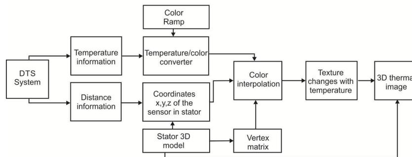
Fig. 2. Block diagram of the thermal imaging of generator stator using DTS system.
