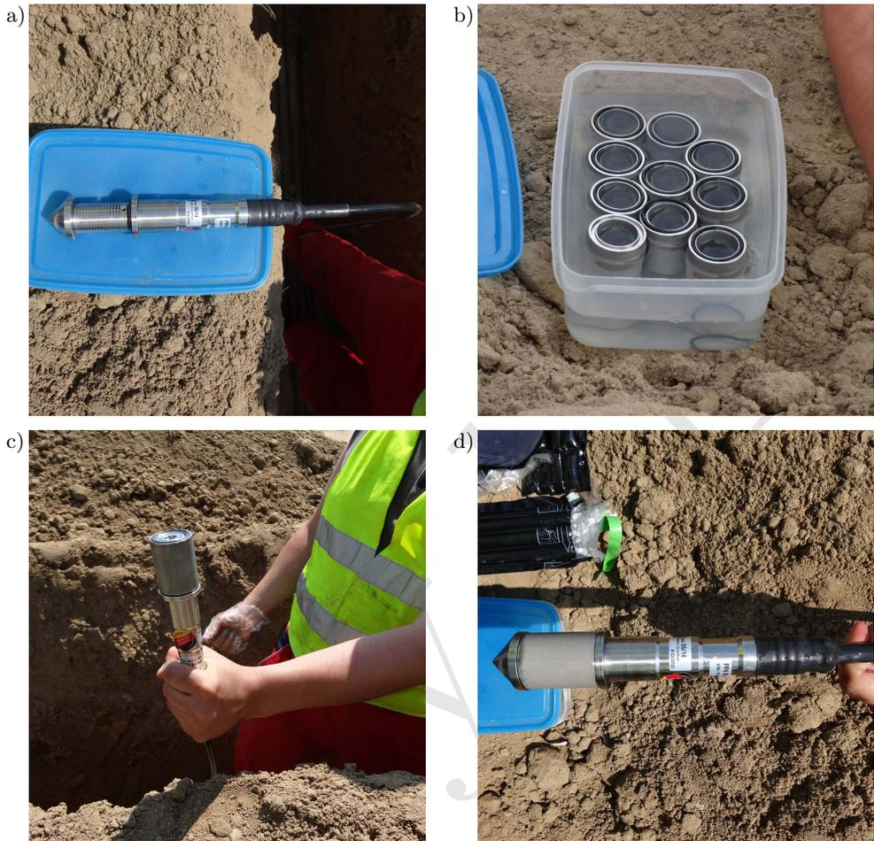
**Figure 3.** Installation of porometer: A – sensor prior to the installation of the filter, B – filters prior to the installation, C – filter installation, D – sensors after the installation of the filter [8].
