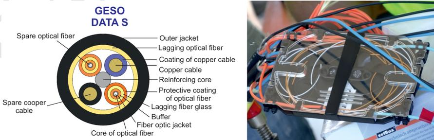
Figure 6. Cross-section of fiber-optic cable and its installation in levee [8].
