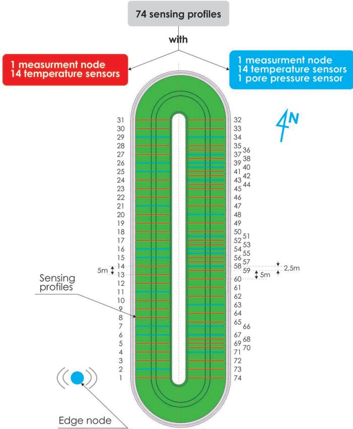
Figure 10. Location of sensing profiles in experimental levee.
