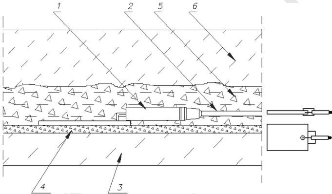
**Figure 4.** Installation diagram for pressure pad sensors: 1 – sensor EE VW 20/30 K2 C; 2 – cable PE 4x0.5 ; 3 – underlayer of earth; 4 – sand bed, 5 – wet, fine earth; 6 – next layers of earth [8].
