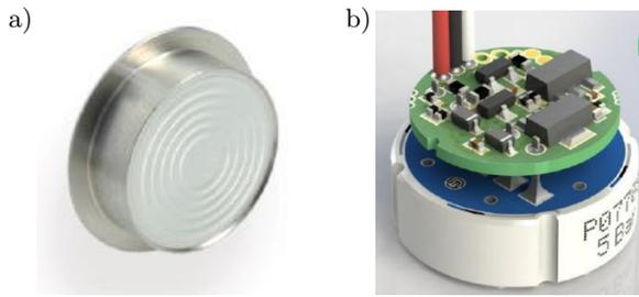
**Figure 16.** Pressure sensor chips applied in the experiment: A – Keller-Druck chip Paa-9FLD ( $\varnothing 17$  mm), B – Metallux chip ME 722 ( $\varnothing 18$  mm).
