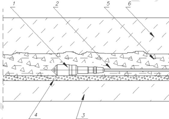
**Figure 2.** Porometer installation diagram: 1 – sensor PP4 RS VW 0.7, 2 – cable PE 4×0.5, 3 – underlayer of earth, 4 – sand bed, 5 – wet, fine earth, 6 – next layers of earth [8].
