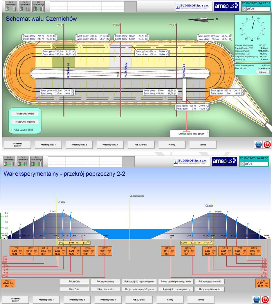
Figure 8. The SCADA system screens.
