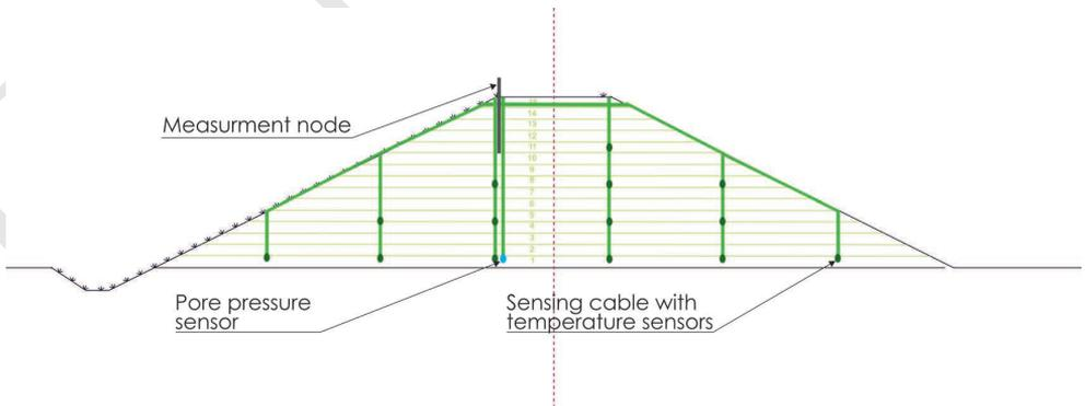
Figure 11. Scheme of installation point of temperature sensors.
