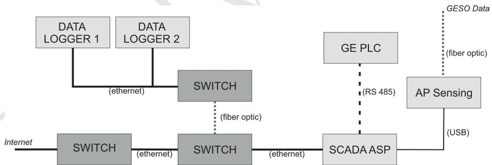
**Figure 7.** Detailed diagram of Automatic Measurement System (ASP).
