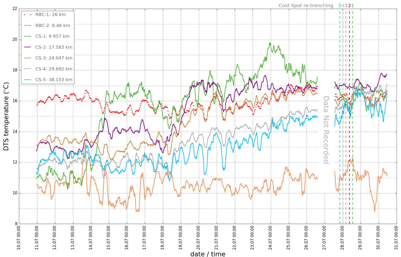
**Fig. 5: DTS time series (10-31/07 2018) for Cold Spot positions CS-1 to CS-5 and Reference Buried Cable sections at 8.46 km and 26 km. The timing of the re-trenching operations (starting at CS-5) is also indicated**
