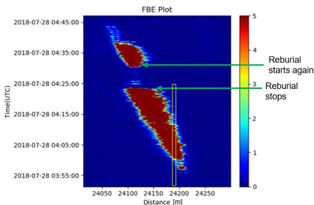
**Fig. 4: An example of the Distributed Acoustic Sensor data for Cold Spot 3 (CS-3) during reburial**
