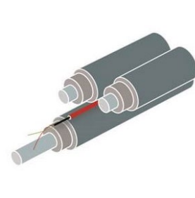
Figure 1: Setup of FOC with power cable
