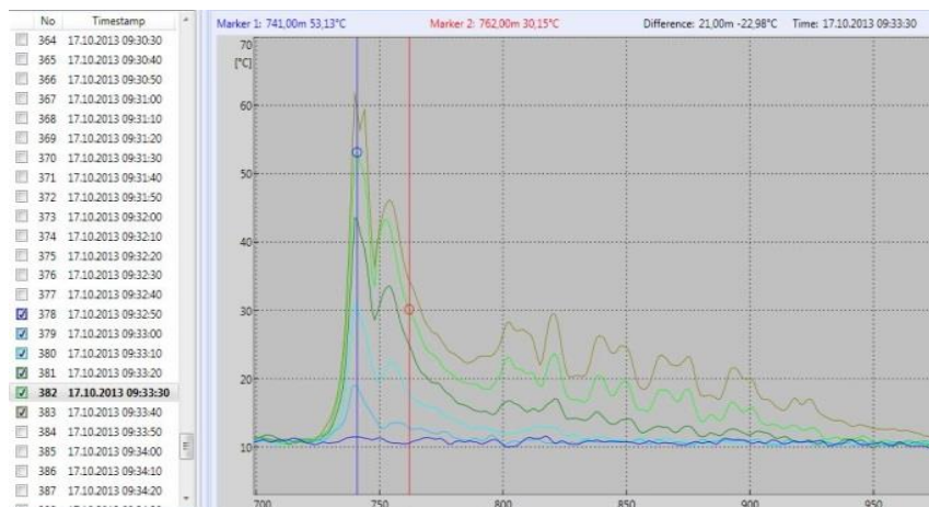
Test 2 (Petrol fire): 5 MW ; Detection time: 33 s
