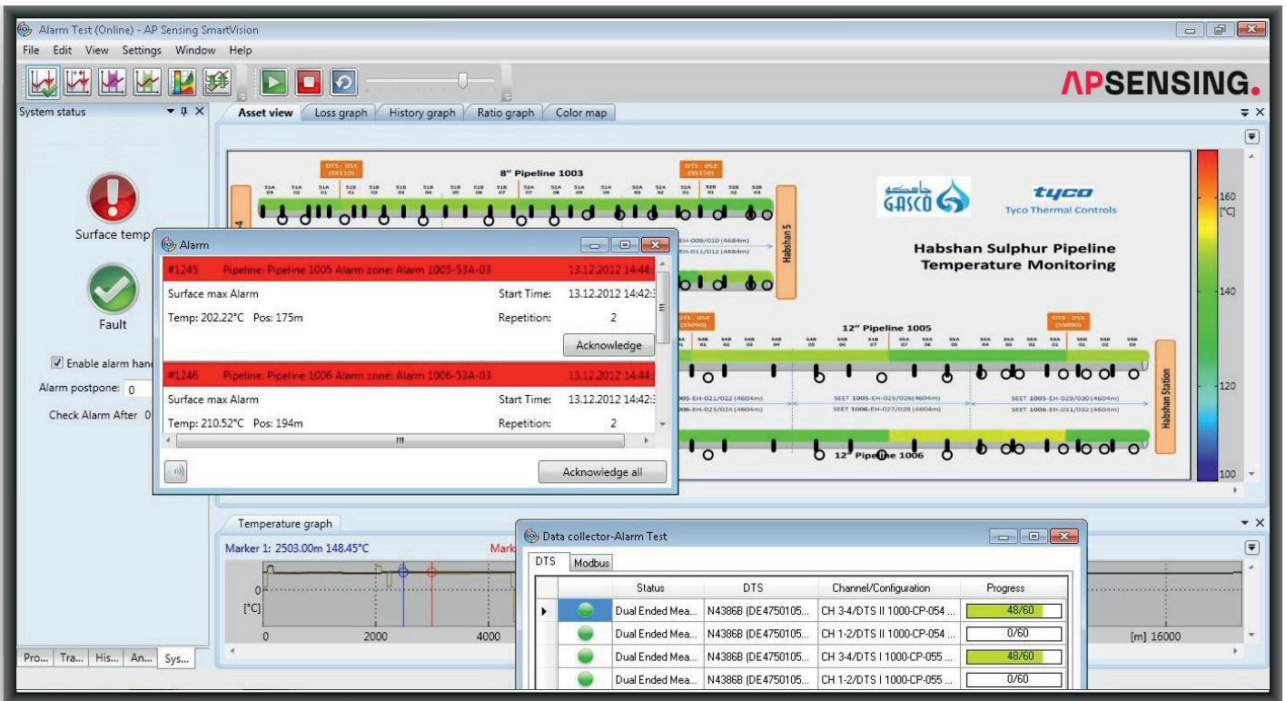
Figure 1: SmartVision Trace details of a heated pipeline
