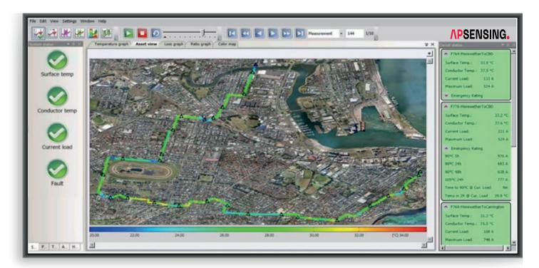
operator was able to adjust his steady state load table by +14%. Additionally, it shows that load could be increased by 32% if a temperature of 90 °C is tolerated for 24 hours. If a temperature of 105 °C is tolerated for 24 hours during peak loads or emergencies, a 48% capacity increase can be realized.
