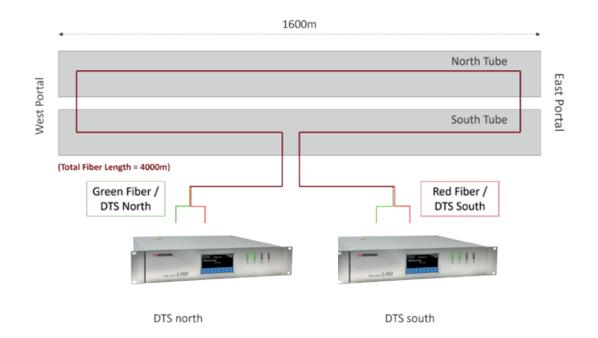
This solution for fire detection is highly suitable for longer tunnels, as the LHD system can monitor the tunnel along the entire length of the sensor cable and the fiber is more cost effective compared to alternative methods. Furthermore, the LHD enables greater flexibility, as individual zones in the tunnel can be defined which trigger alarms based on different alarm parameters. In this tunnel, 25 different alarm zones were configured and one output relay was assigned to each zone.
