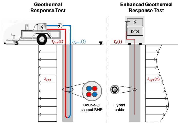
Figure 1. Schematic comparison of GRTs and EGRTs.
