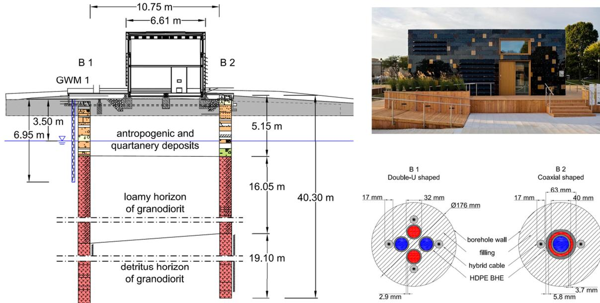
**Figure 2. Drilling log and cross section of B 1 and B 2.**
