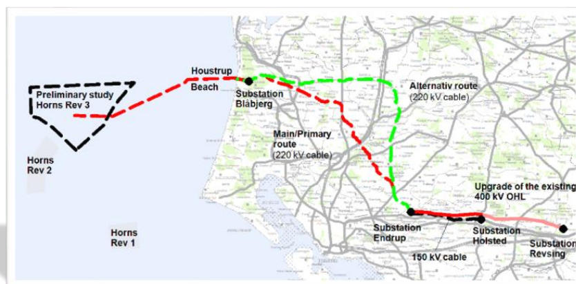
Off- and onshore power cable routing
