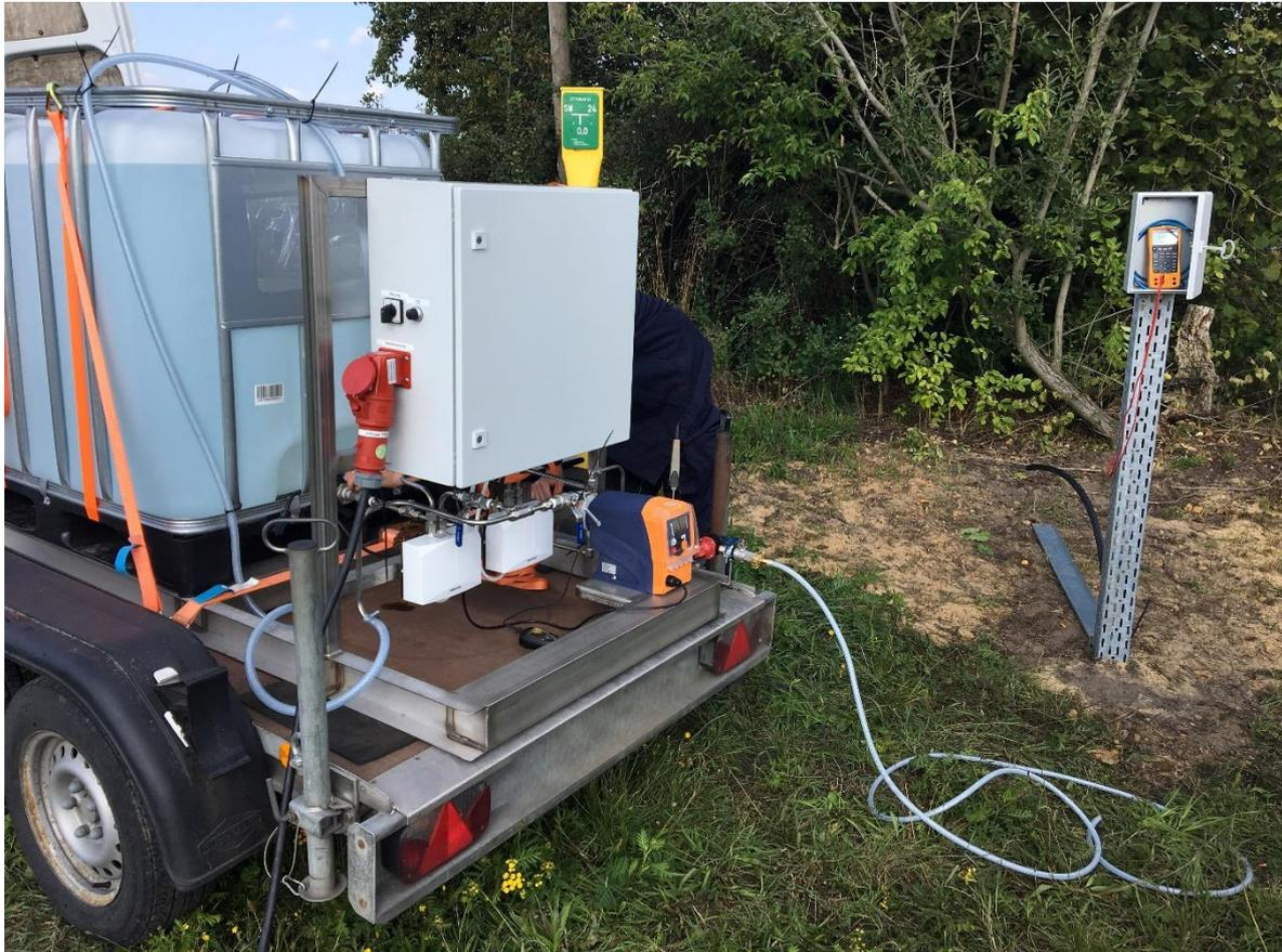
*Leak detection test vehicle*
