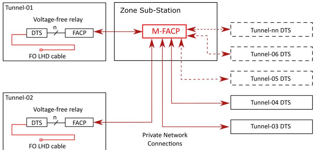
Each cable tunnel has been divided into individual fire detection zones, enabling the LHD to report the accurate location of a fire event to the FACP in real time. The systems were configured appropriately to ensure compliance to UL 521 and FM 3210 regulations.
