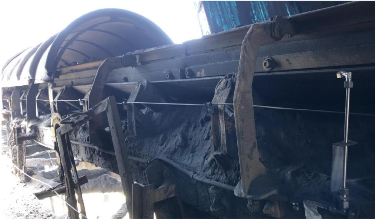
*Copper conveyor belt with sensor cable at Ventanas Operation*
